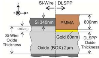
Fig.2. Side-view of the DLSPP-to-Silicon interface layout.
