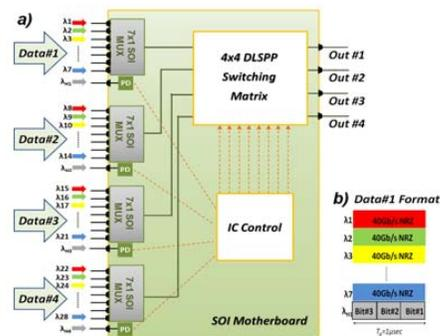
Fig.1. a) The architecture of PLATON's 4x4 Tb/s routing fabric and b) the multiwavelength data packet format.
