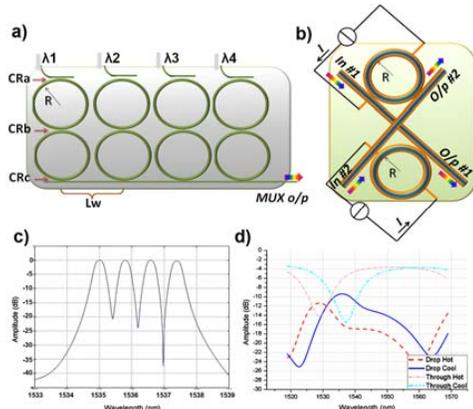
Fig.3. a) 4:1 SOI MUX design, b) 2x2 PMMA-loaded SPP switch, c) 4:1 SOI MUX transfer function, and d) SPP switch transfer function.
