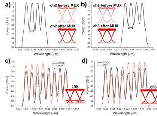
Fig.5. a) and b) Outputs of the two SOI MUX devices, c) and d) multiwavelength signal obtained at the switch outputs #1 and #2, respectively, both for the case of unheated and heated states. Inset in a), b) show the eye diagrams of ch2 and ch6 before and after the SOI MUX, respectively, and inset in c) and d) show the eye diagram of ch6 at the respective switch outputs.
