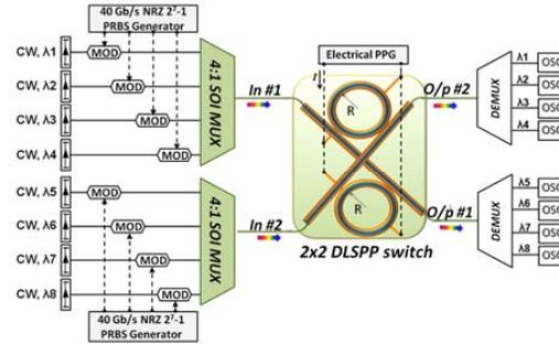
Fig.4. Layout of the 2x2 silicon-plasmonic 320Gb/s router.
