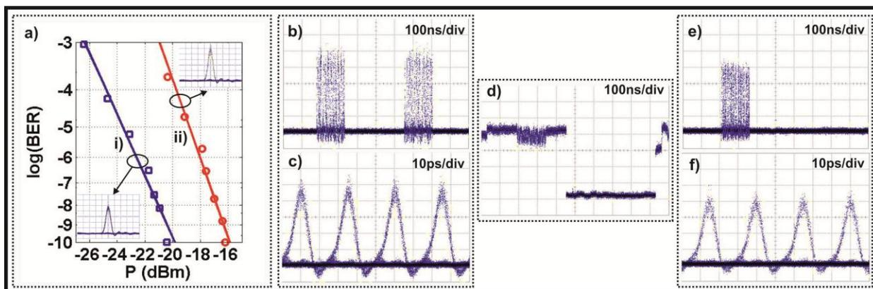
Figure 3: a) BER curves of i) input packets, ii) forwarded packet b) input packets trace c) 40 Gb/s input data eye-diagram d) Flip-flop state (port7) e) forwarded packet trace f) 40 Gb/s forwarded packet eye-diagram.
