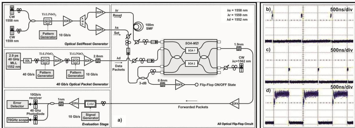
Figure 2: a) Experimental setup b) Set pulses c) Reset pulses d) Flip-flop response with no data signal.
