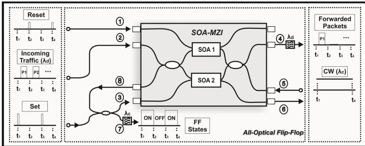
Figure 1: Conceptual diagram of forwarding gate setup.
