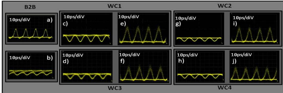
**Figure 3:** Eye-diagrams of a) B2B signal, b) SOA recovery, c),g),d),h) Inverted signals at the output of WC1, WC2, WC3, WC4, e),i),f),j) Non-Inverted signals at the outputs of WC1, WC2, WC3, WC4 respectively.
