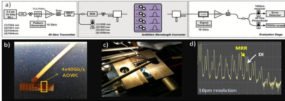
Figure 2: a) Experimental setup, b) TriPlex™ chip, c) Fiber and probe alignment, d) MRR and DI spectral responses in case of ASE seed
