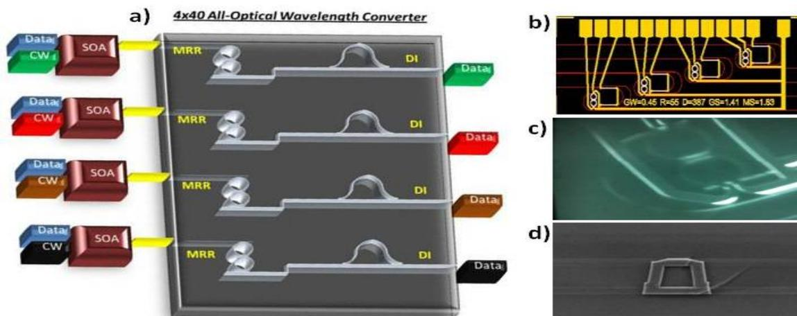
Figure 1: a) Concept of 4x40 AOWC, b) Mask of TriPleX™ chip, c) 2<sup>nd</sup> Order Ring Resonator View, d) SEM of TriPleX™ Waveguide
