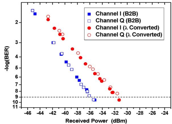
Fig. 7. BER curves for the back-to-back and the converted QPSK signals.
