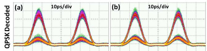
Fig. 4. Decoded signals after the (a) upper and (b) lower 22-GHz DI.
