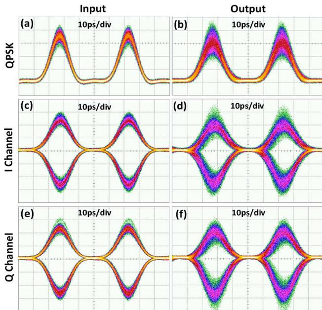
Fig. 6. Signals at the input (left column) and output (right column) of the wavelength converter: (a), (b) QPSK signals, and corresponding decoded (c), (d)  $I$ -channels and (e), (f)  $Q$ -channels detected with the balanced detector.
