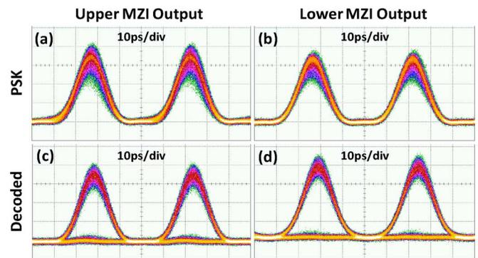
Fig. 5. PSK signals at the output of the (a) upper and (b) lower SOA-MZI, and (c), (d) the corresponding decoded signals.
