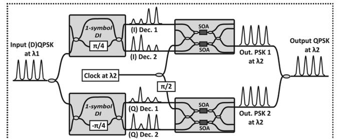
Fig. 1. Operating principle of the (D)QPSK wavelength-converter.
