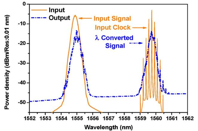
Fig. 3. Spectra at the input and output of the MFPC-based  $\lambda$ -converter.
