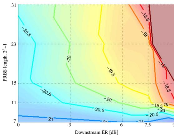
Fig. 5. (Color online) Upstream reception sensitivity for a BER of  $10^{-9}$  as a function of the downstream ER and the PRBS length. The dark area top right indicates a BER floor above  $10^{-9}$ .
