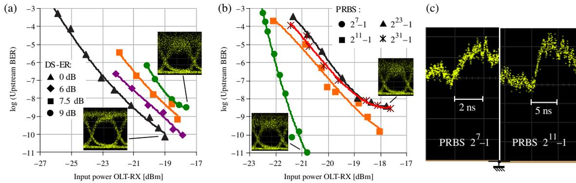
Fig. 4. (Color online) Upstream BER for (a) a PRBS of  $2^{31}-1$  and different downstream ERs, and (b) a fixed downstream ER and different PRBS lengths. (c) Recovered optical carrier after the FPF for the case of experiencing the largest number of consecutive identical mark bits inside the PRBS.
