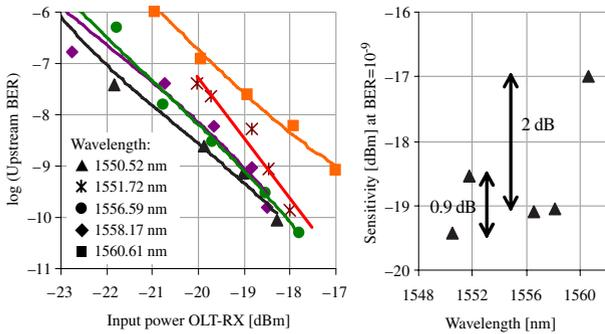
Fig. 7. (Color online) Upstream BER for different downstream wavelengths and the corresponding reception sensitivity spectrum for a BER of  $10^{-9}$ .
