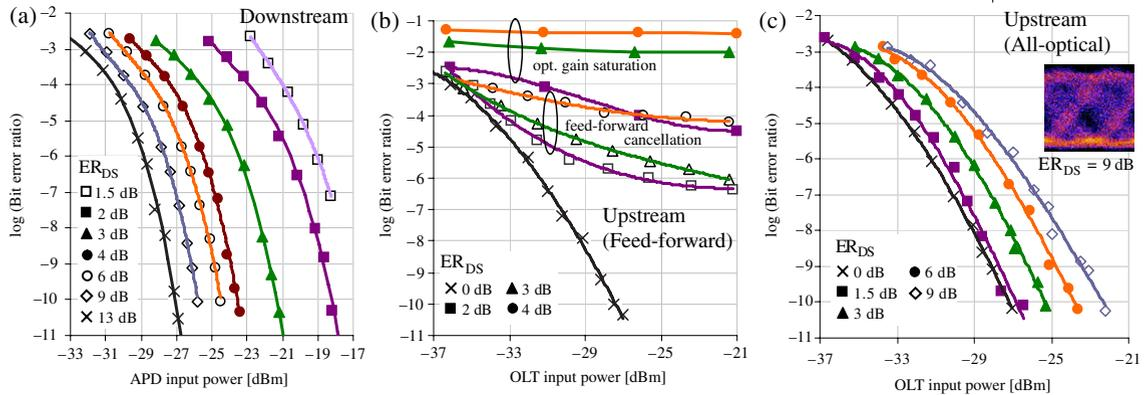
Fig. 3. (Color online) BER performance for (a) the downstream and the upstream including (b) a feed-forward and (c) an all-optical carrier recovery technique.
