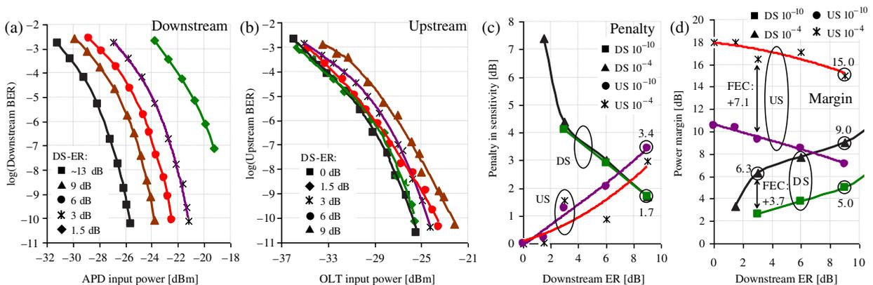
Fig. 9. (Color online) BER measurements for (a) the downstream and (b) the upstream. (c) Reception penalties, referenced to an ER of 13 dB for the downstream and to an ER of 0 dB for the upstream. (d) Power margins with and without FEC.
