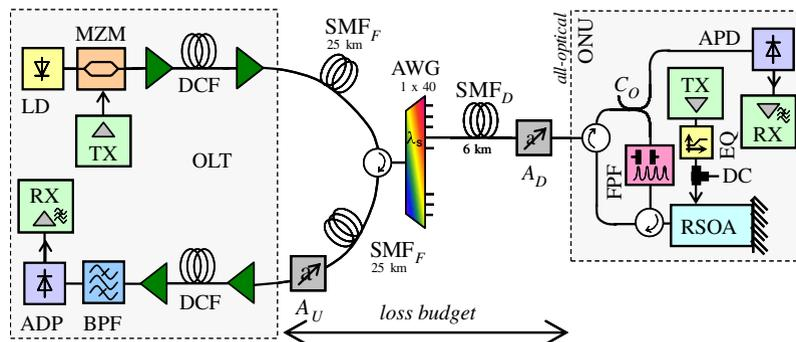
Fig. 8. (Color online) Experimental setup for evaluating the all-optical carrier recovery in a WDM-PON with bidirectional 10 Gb/s data transmission on a single wavelength.
