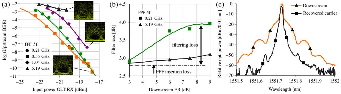
Fig. 6. (Color online) (a) Upstream BER for a PRBS of  $2^{11} - 1$  and a downstream ER of 9 dB for different FPF bandwidths, (b) the FPF loss and (c) the signal spectra for the incident downstream and the recovered carrier, whose optical power levels are referenced to that of the optical carrier wavelength at 1551.72 nm of the downstream.
