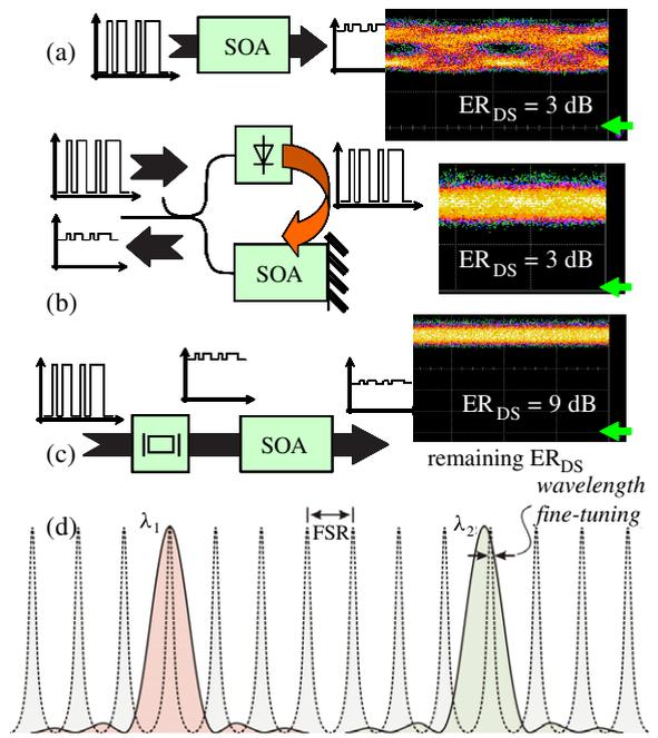
Fig. 1. (Color online) Pattern suppression techniques based on (a) optical gain saturation in a SOA, (b) feed-forward current injection and (c) passive optical resonating circuit. The insets on the right show the recovered optical carriers, for which the arrows indicate the reference levels. (d) WDM operation of the all-optical carrier recovery with FPF. Periodic filter peaks (dotted line) coincide with the downstream wavelength grid.
