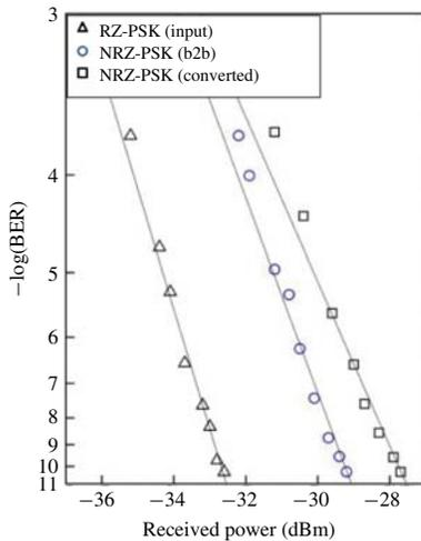
Fig. 6. BER curves for the input RZ-PSK, the converted NRZ-PSK, and the back-to-back (b2b) NRZ-PSK signal.
