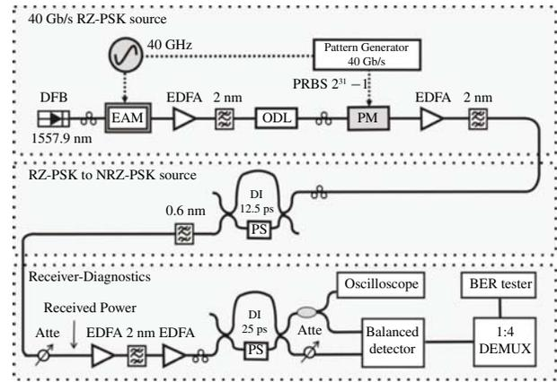
Fig. 4. Experimental setup for the RZ-to-NRZ conversion of DPSK signals.
