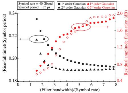
Fig. 3. Rise/fall times (10%–90%) of the intensity dips and residual amplitude fluctuation of the converted NRZ-DPSK signal as a function of the OBPF. Normalized values are used for the rise/fall times and the filter bandwidth.
