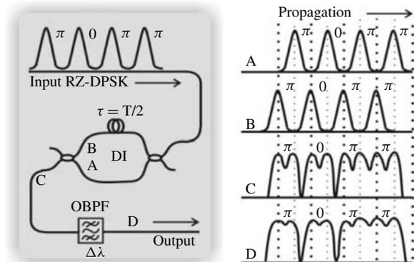
Fig. 1. Concept of RZ-to-NRZ conversion in the case of a DPSK signal.
