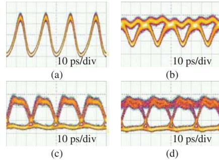
Fig. 5. Experimental results. Eye-diagrams of (a) input RZ-PSK signal, (b) converted NRZ-PSK signal, and (c)–(d) corresponding decoded streams.
