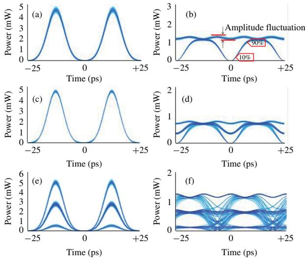
Fig. 2. Simulation results (eye-diagrams) for 40 Gbaud modulated signals (a)–(b) input RZ- and converted NRZ-DPSK signals, (c)–(d) input RZ- and converted NRZ-DQPSK signals, and (e)–(f) input RZ- and converted NRZ-16-QAM signals. The duty-cycle of all input signals is 33%.
