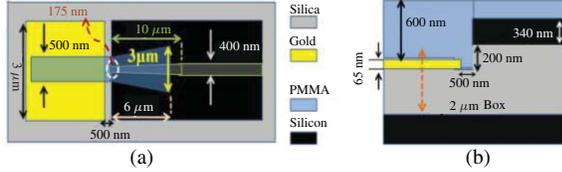
Fig. 2. Schematic of DLSP to Si-rib waveguide transition: (a) top and (b) side view.
