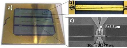
Fig. 1. (a) Real view of Si-Plasmonic chip. (b) Microscope image of the 60- $\mu\text{m}$ -long DLSP waveguide. (c) SEM image of an ll-pass racetrack ring resonator.
