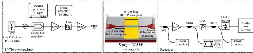
Fig. 4. Experimental setup of the 10-Gb/s transmission experiment through the straight DLSP waveguide.
