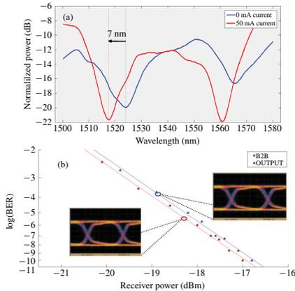
Fig. 5. (a) Spectral response of racetrack ring resonator over the range of 1500–1580 nm. (b) BER measurements and eye diagrams of the B2B and the output signal transmitted through the 60- $\mu\text{m}$  Si-DLSP waveguide.
