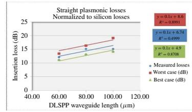
Fig. 3. Cutback measurements on 60-, 80-, and 100- $\mu\text{m}$ -long DLSP waveguide samples.
