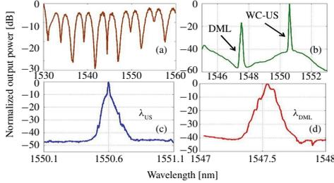
Fig. 3. Spectra of (a) cascaded DI response in case of ASE injection, (b) output of AOWC, (c) WC US, and (d) DML output.
