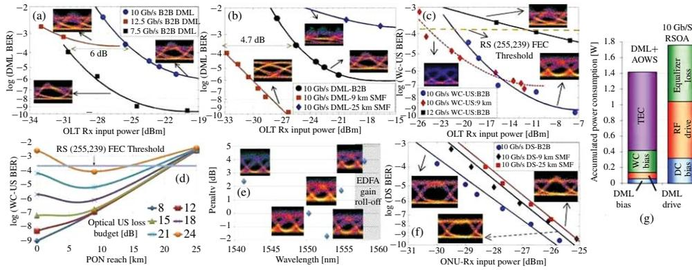
Fig. 4. (a) and (b) BER for DML-US in (a) B2B and different rates and (b) transmission at 10 Gb/s. (c)–(e) BER for WC-US at (c) different rates, (d) different PON reach, and (e) for colorless operation. (f) BER for DS at 10 Gb/s. (g) Power consumption comparison for the AOWC- and a RSOA-based ONU.
