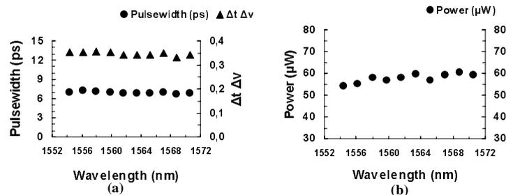
Fig. 3. (a) Variation of the pulsewidth and pulsewidth-bandwidth product vs wavelength, (b) Variation of the output power vs wavelength.
