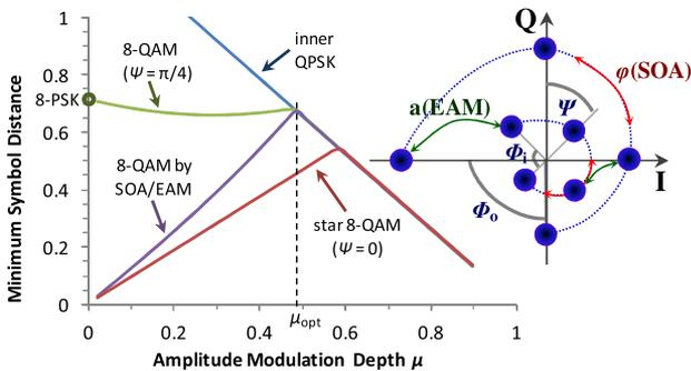
Fig. 1. (Color online) Phasor diagram for the generation of octary QAM with an SOA/EAM and resulting minimum symbol distance as function of the amplitude modulation depth.
