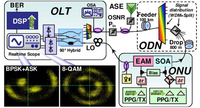
Fig. 2. (Color online) Experimental setup for the performance characterization of the m-QAM transmitter in coherent PONs.
