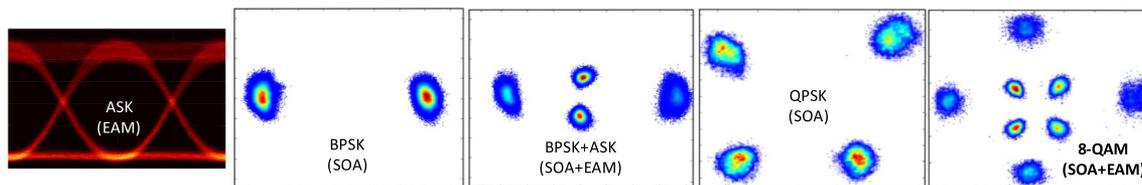
Fig. 4. (Color online) Multifformat generation with SOA + EAM: constellations for ASK, BPSK, BPSK + ASK, QPSK, 8-QAM.
