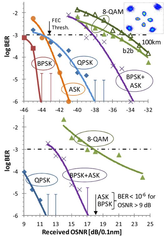
Fig. 3. (Color online) BER for ASK, BPSK, QPSK, PSK + ASK and 8-QAM as function of input power (for fixed OSNR of 41 dB for all back-to-back measurements) and as function of the delivered OSNR (for fixed input power of -32 dBm).
