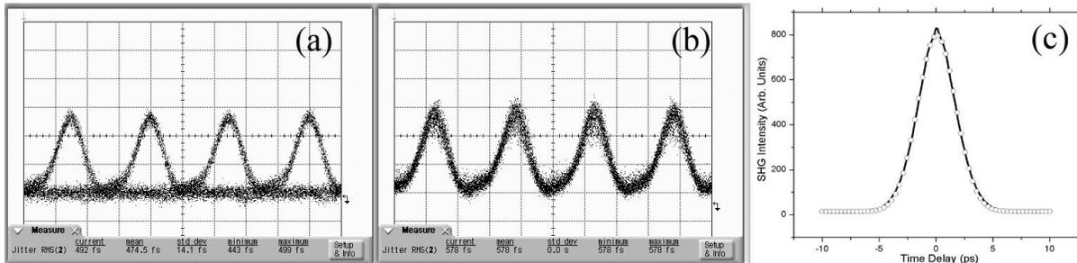
Fig. 3. (a), (b) Eye diagrams (100ps/div, 500  $\mu$ W/div) of input data and extracted clock and (c) Autocorrelation trace and sech fit of clock pulses.
