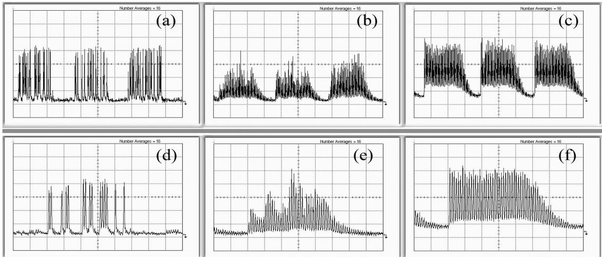
Fig. 2. (a), (b), (c) Input data packets, FPF output and recovered clock packets (time base 500 ps/div, vertical scale 335  $\mu$ W/div) and (d), (e), (f) Single packet, FPF output and recovered clock (time base 200 ps/div, vertical scale 335  $\mu$ W/div)
