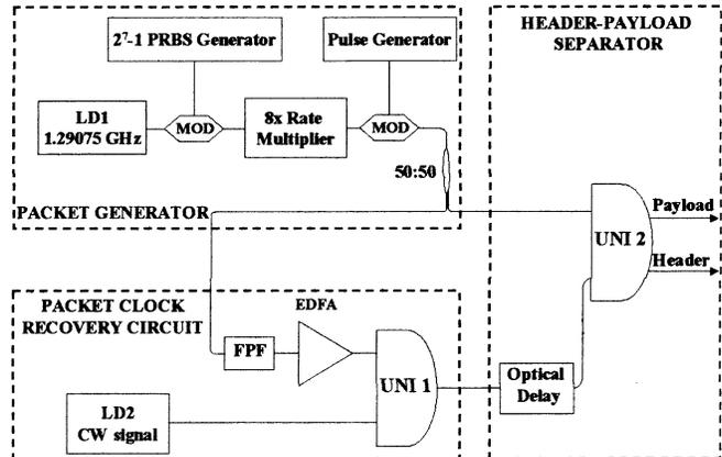
Fig. 1. Block diagram of the all-optical address and payload separation circuit.
