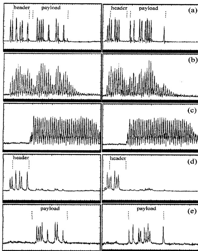
Fig. 3. (a) Typical data packets. (b) Corresponding output from the FP filter. (c) Recovered and delayed packet clock. (d) Packet address at U-port. (e) Packet payloads at S-port of UNI 2. The time base is 500 ps/div.
