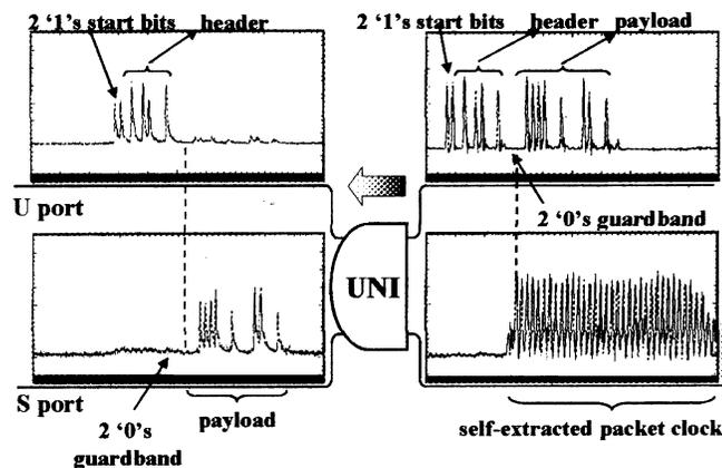
Fig. 2. Principle of operation of header/payload separation.
