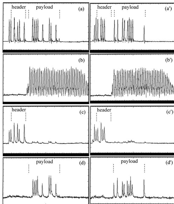
Figure 3:(a), (a') Typical data packets, (b), (b') corresponding recovered packet clock at exit of UNI 1, (c), (c') packet address at U-port and (d), (d') packet payloads at S-port of UNI 2. The time base is 500 ps/div.
