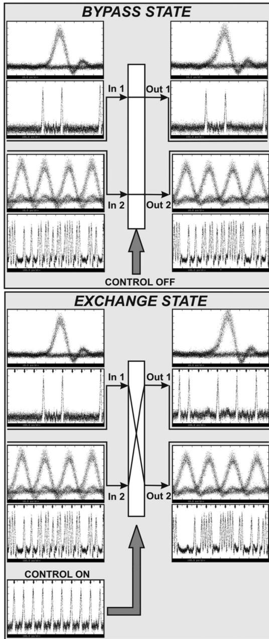
Fig. 2. Oscilloscope traces and respective eye diagrams in the BYPASS and EXCHANGE states. First column: BYPASS state operation. Second column: EXCHANGE state operation. The time base is 100 ps/div for the oscilloscope traces and 10 ps/div for the eye diagrams. Arrows indicate the time slots which coincide with the control pulses.
