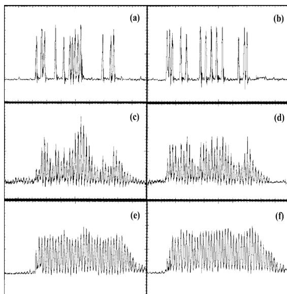
Figure 2 (a), (b) Two different data packets, (c), (d) Corresponding outputs from the FP filter (e), (f) Output of the UNI gate for both packets. The time base is 500 ps/div
