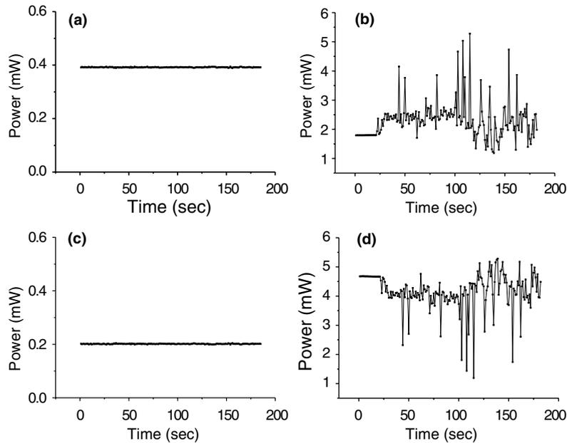
Fig. 4. Power vs. time at (a) transmit and (c) reflect port using the polarization insensitive NOLM and (b) transmit and (d) reflect port of a conventional NOLM. All the measurements were recorded in the presence of an external vibration source.
