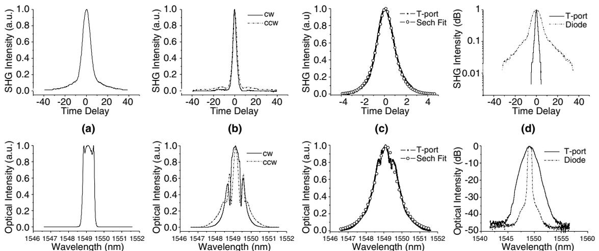
Fig. 3. Intensity autocorrelation traces (upper row) and optical spectra (bottom row) of the: (a) Input signal. (b) Signals after the 1st stage of compression (CW, clockwise; CCW, counter-clockwise). (c) Transmitted signal in linear scale and ideal sech fit. (d) Signal after DCF and transmitted signal in logarithmic scale.
