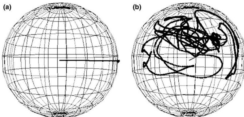
Fig. 5. Poincaré spheres at the transmit port of (a) the polarization insensitive NOLM and (b) conventional NOLM compressor.
