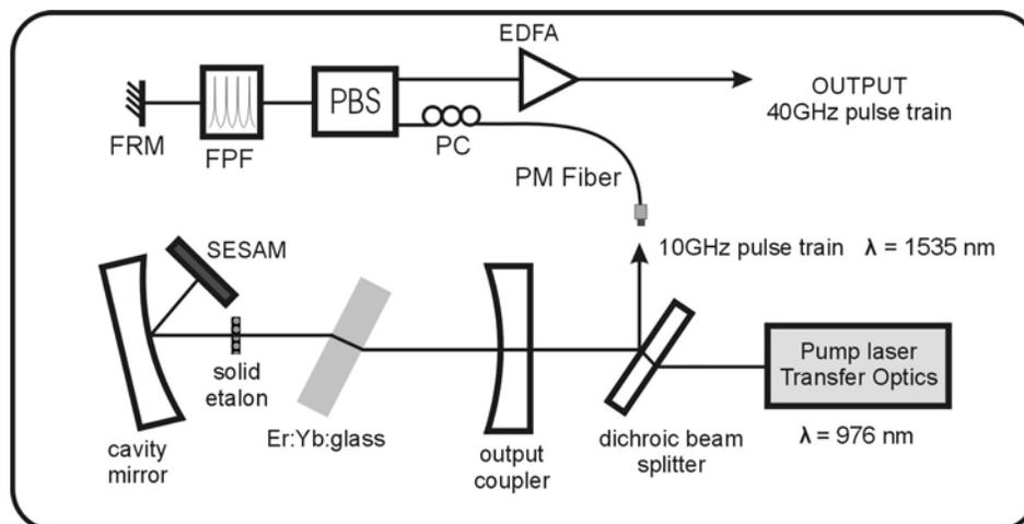
Fig.1 Schematic diagram of the experimental layout.
