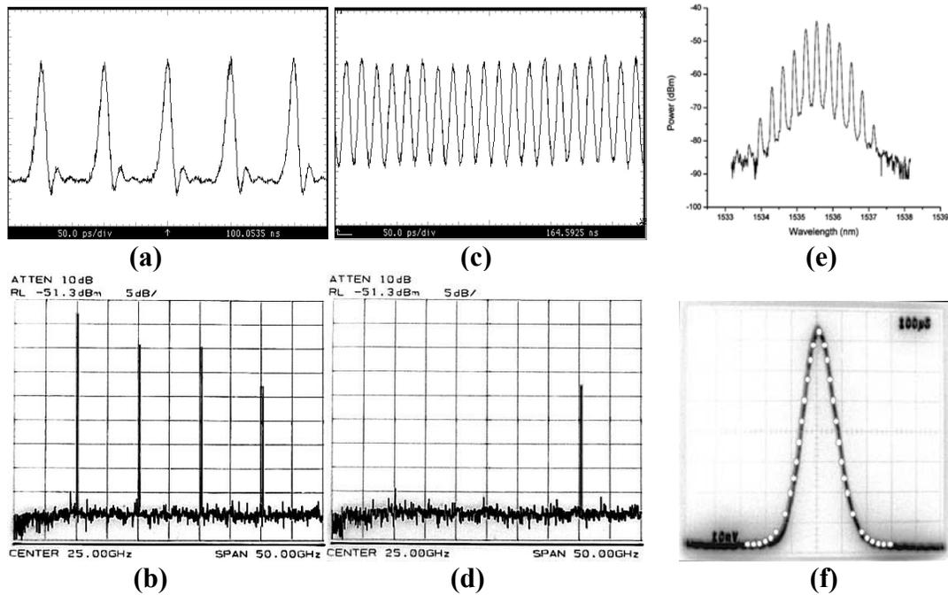
Fig.2 Experimental results including the pulse traces and microwave spectra of 10 GHz pulse train (a), (b) and 40 GHz pulse train (c), (d), respectively. (e) shows the optical spectrum of 40 GHz pulse train and (f) the autocorrelation trace of the laser source fitted on a hyperbolic secant profile.
