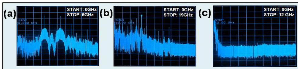
Fig. 2: Electrical spectra of signals. (a) After up-conversion and combination. (b) After receiver. (c) After LPF.
