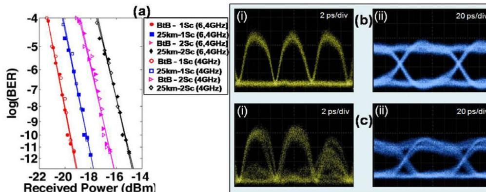
Fig. 3: (a) BER curves at BtB and 25km transmission for single and 2 sub-carrier multiplexing. Optical eye diagrams at 25km transmission for (b) single sub-carrier multiplexing and (c) 2 sub-carrier multiplexing.
