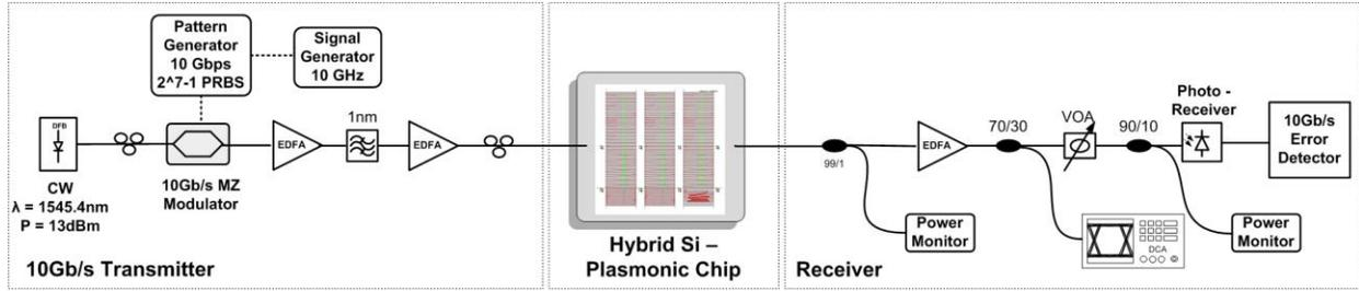
**Figure 2:** Experimental Setup of the 10Gb/s transmission experiment through the straight DLSP waveguide
