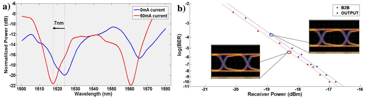
**Figure 3:** (a) Spectral Response of racetrack ring resonator over the range of 1500 - 1580nm, (b) BER measurements and Eye Diagrams of the B2B and the transmitted, through the 60um Si-DLSPP waveguide, signal
