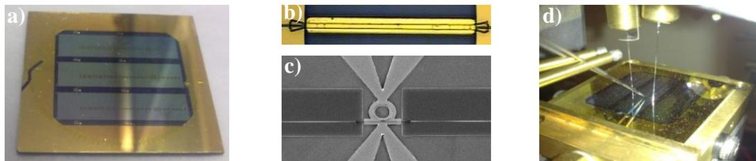
**Figure 1:** (a) The hybrid Si - Plasmonic chip, (b) Straight DLSPP waveguide of 60um, (c) All - Pass Racetrack Ring Resonator, (d) Chip on Probe Station
