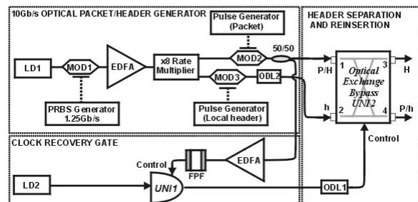
Figure 1. Simplified Experimental Setup
