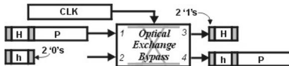
Figure 2. Concept and bit synchronisation scheme
