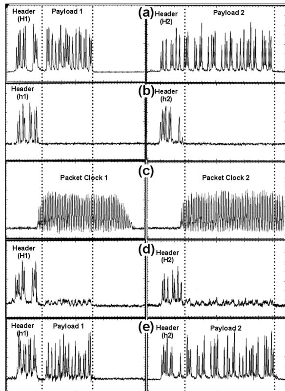
Figure 3. Experimental results for 4.4 ns and 6.6 ns packets. The timebase is 800 ps/div.
