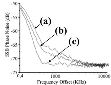
Fig. 3. SSB spectra at 40GHz of (a) input, (b) received output data and (c) recovered clock
