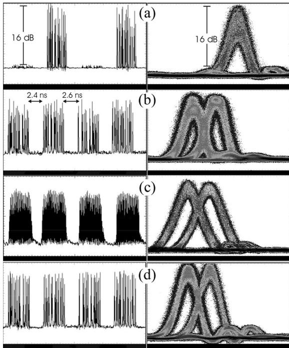
Figure 2: Oscilloscope traces (2.5 ns/div) and eye diagrams (10 ps/div) of (a) bursty packets, (b) equalized packets, (c) recovered clock packets and (d) received packets
