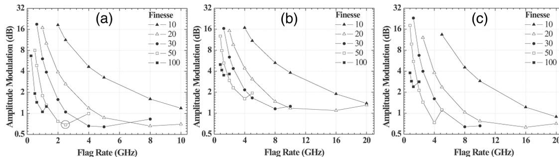
Fig. 3. Calculated amplitude modulation versus the flag repetition rate for several FP filter finesses when the line rate is (a) 40 GHz and (b) 80 GHz and a SOA with 65-ps recovery time is employed. The circle indicates the experimental point. (c) Same as (b), but with a SOA with a 20-ps recovery time.
