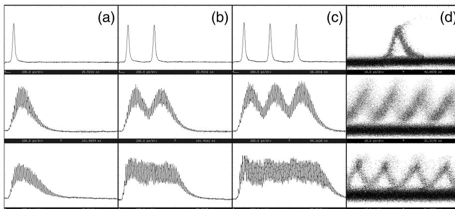
Fig. 2. Oscilloscope traces for (a) one, (b) two, and (c) three flags. The rows correspond to the flag pulses, the output of the double-pass FP filter, and the generated control signals at the output of the SOA. Time base is 200 ps/div. (d) Equivalent pulse waveforms. Time base is 10 ps/div.
