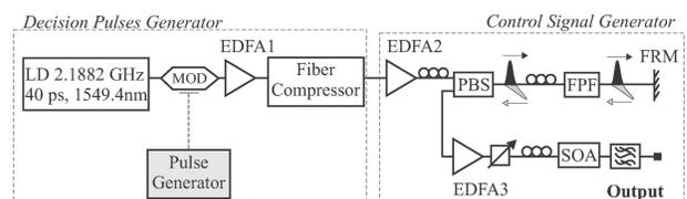
Fig. 1. Experimental setup: LD, laser diode; MOD, modulator; PBS, polarization beam splitter; FPF, Fabry–Perot filter; FRM, Faraday rotator mirror.
