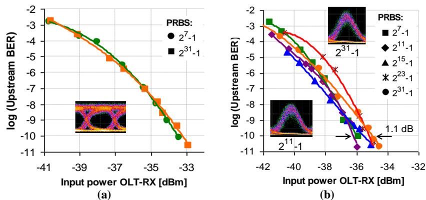
Fig. 3. Upstream back-to-back BER measurements for (a) continuous-wave light seed and NRZ modulation and (b) concurrent RZ downstream clock extraction.
