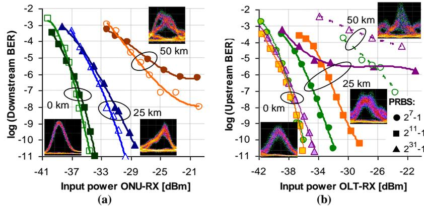
Fig. 4. BER performance for transmission over 25 and 50 km fiber spans in case of (a) the downstream (filled and hollow markers indicate a PRBS  $2^{31}-1$  and  $2^7-1$ , respectively), and (b) the upstream that uses the recovered downstream clock as optical seed.
