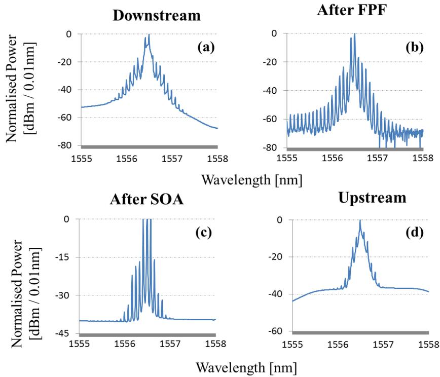
Fig. 2. Spectra of different ONU signals after 50 km transmission. a) Downstream, b) after the FPF, c) after passing through the SOA and d) upstream.
