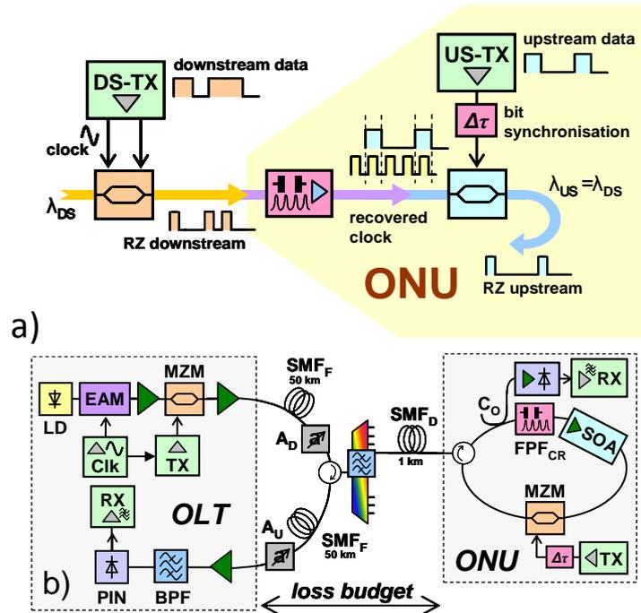
Fig. 1. (a) Colorless ONU design based on remodulation of the recovered clock from downstream transmission, (b) experimental setup.
