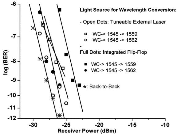
Fig. 5. BER measurements for static flip-flop operation.
