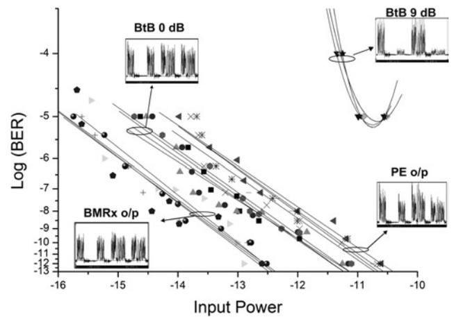
**Fig. 3** Experimentally measured BER results at various parts of the BMR circuit
