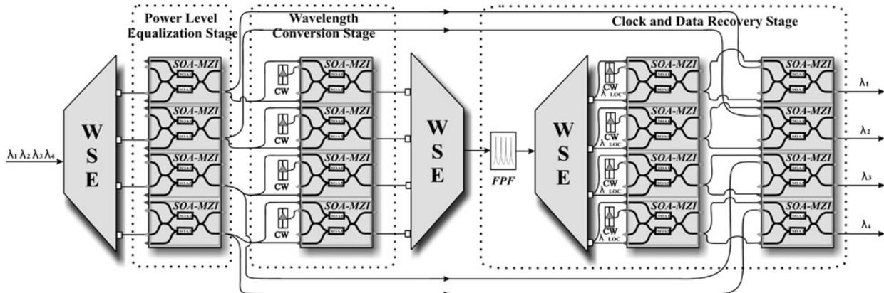
**Fig. 5** Schematic design of the four-channel burst-mode receiver using the integrated quadruple switch arrays
