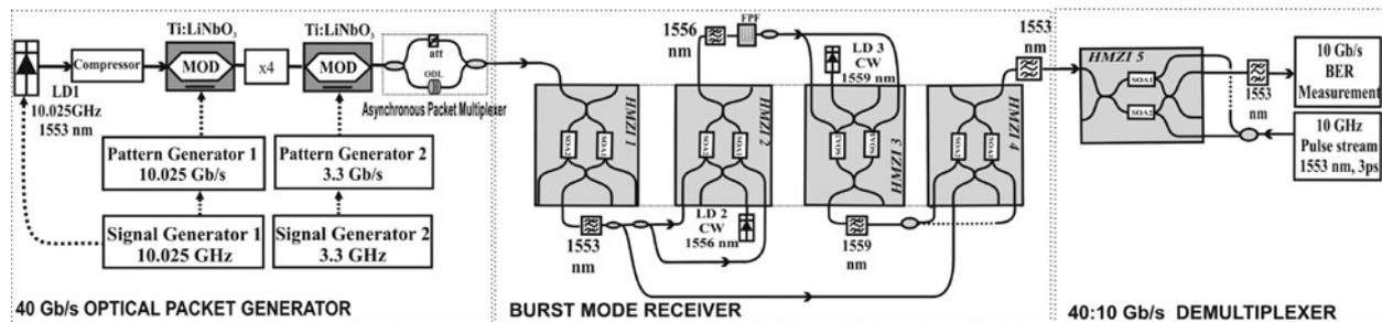
**Fig. 1** Experimental setup. HMZI1 operates as a power equaliser, HMZI2 performs wavelength conversion and HMZI3 and HMZI4 are responsible for the clock-and-data recovery process
