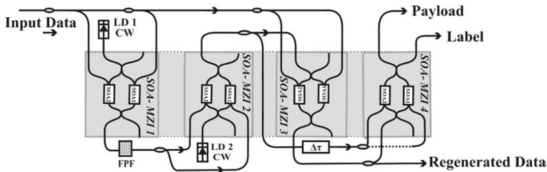
**Fig. 6** Block diagram of the whole front-end unit of an optical packet switched node based on an integrated quadruple switch array. SOA-MZI1 performs wavelength conversion, SOA-MZI2 and SOA-MZI3 are responsible for clock-and-data recovery, and SOA-MZI4 separates the header from the payload
