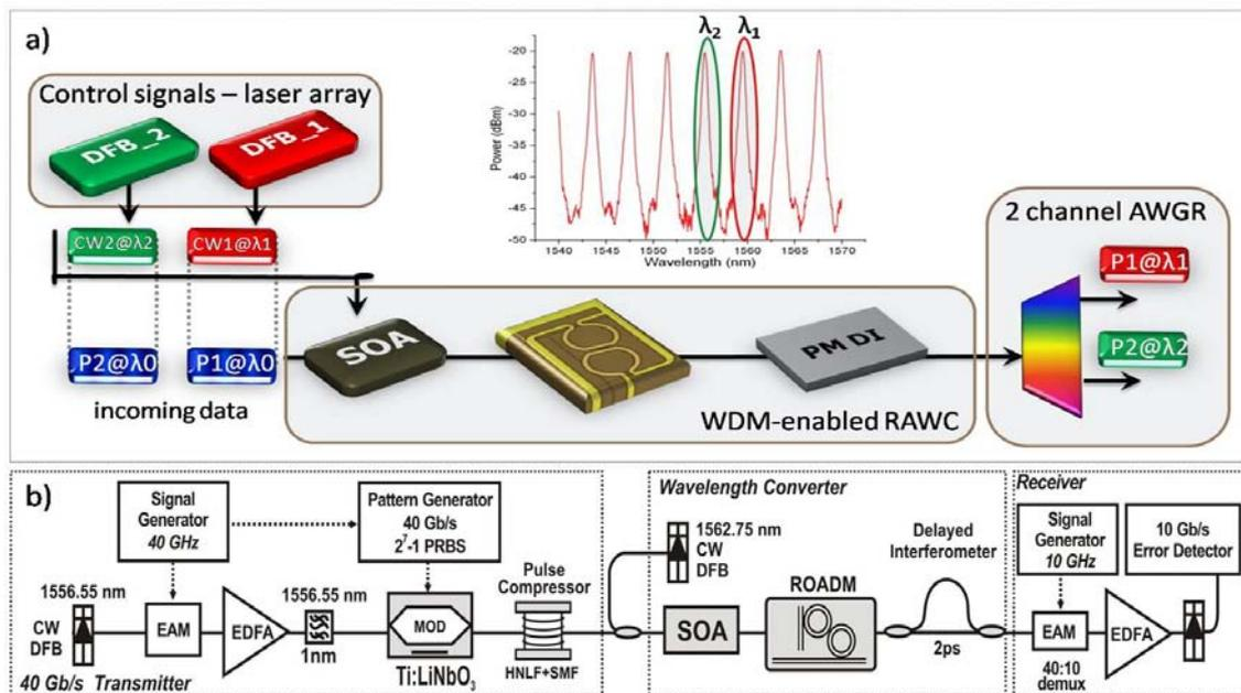
Figure 5 (a) Concept: all-optical wavelength conversion assisted by TriPleX micro-ring resonators, (b) experimental setup for 40 Gb/s continuous-mode wavelength conversion
