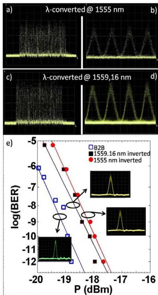
Figure 9. BER curves for RAWC of continuous data
