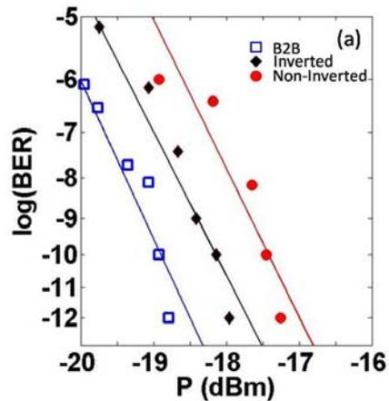
Figure 7. BER curves for RAWC of continuous data
