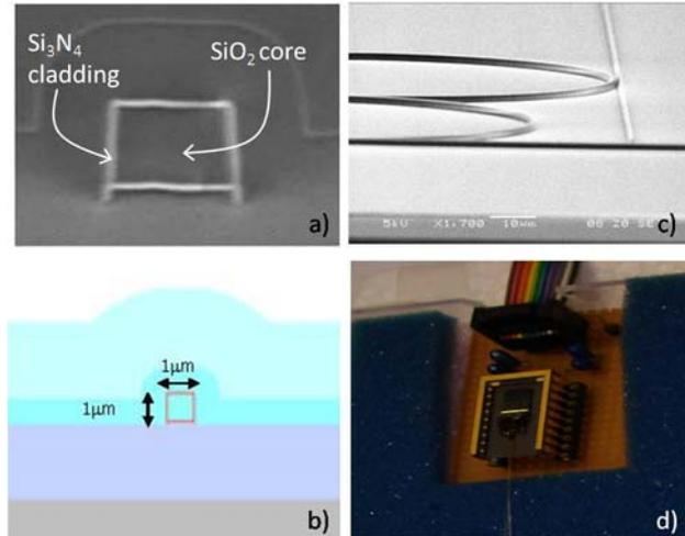
Figure 3. (a) and (b) TriPleX™ waveguide geometry, (c) SEM image of coupled micro-ring resonators, (d) packaged and pigtailed device. Fabrication by LioniX BV, characterization and pigtailling by XiO Photonics BV.
