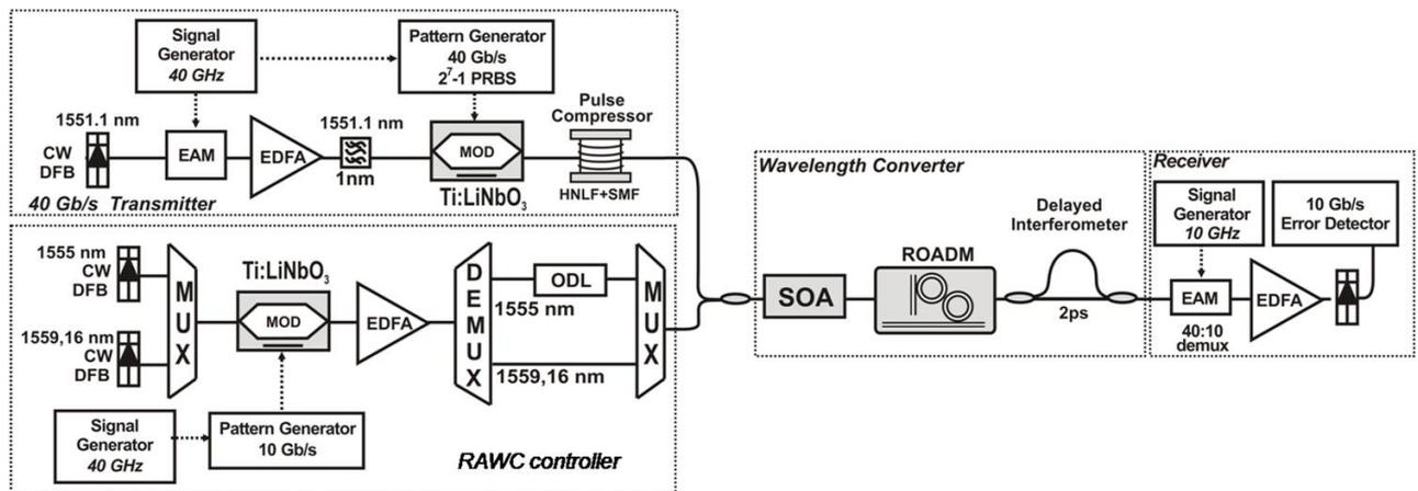
Figure 8. Experimental setup for the packet-mode, WDM-enabled RAWC.
