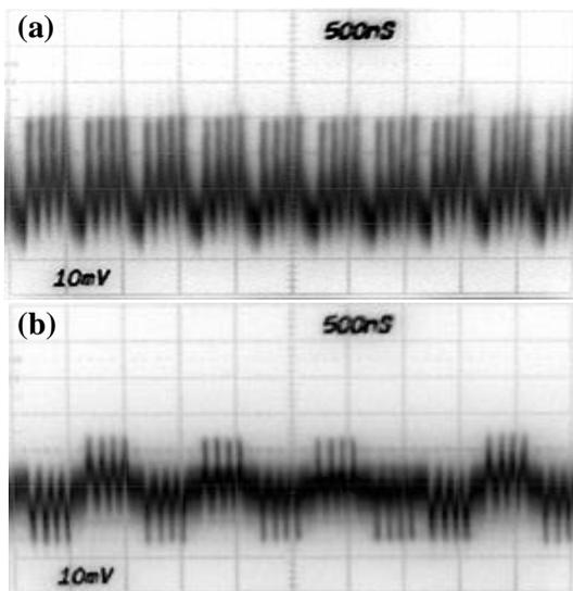
**Figure 2: (a) Memory content with S-port and (b) U port of UNI used in feedback circuit.**
