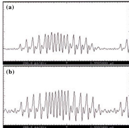
**Figure 3: (a) Loading-up bit sequence and (b) pattern after 7 circulations with S-port in feedback. The time base is 200 ps.**
