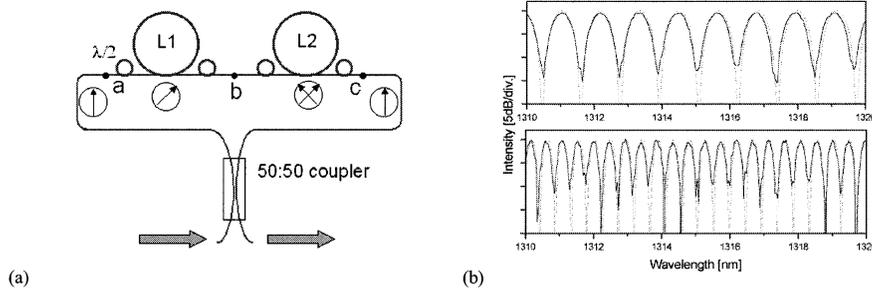
**WJ1 Fig. 2.** (a) Tunable Sagnac loop filter setup. The arrows inside circle represent the relative angle directions of the fast axis of HB fiber and the plane of Sagnac loop. (b) Calculated and measured transfer functions with different wavelength period. The solid lines are for measured transfer function and the dot lines are for calculated transfer function.
