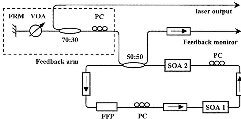
WJ2 Fig. 1. Experimental setup of the multiwavelength laser source.
