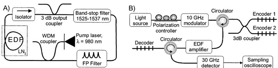
WJ3 Fig. 1. Multiwavelength fiber laser set-up (A) and FFH OCDMA (B).
