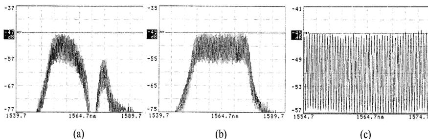
WJ2 Fig. 2. Optical spectrum of the multiwavelength laser (a) without optical feedback; (b) with optical feedback (sweepwidth 5 nm/div); and (c) with optical feedback (sweepwidth 2 nm/div).
