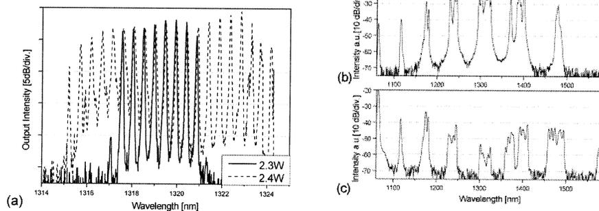
**WJ1 Fig. 3.** (a) Multi-wavelength output spectra of 4th Stokes wave for the pump powers of 2.3 W and 2.4 W. (b) Cascaded Raman spectrum from the output of WDM2 for the pump power of 7.8 W. (c) Cascaded Raman spectrum from the output of WDM1 for the pump power of 8.2 W.
