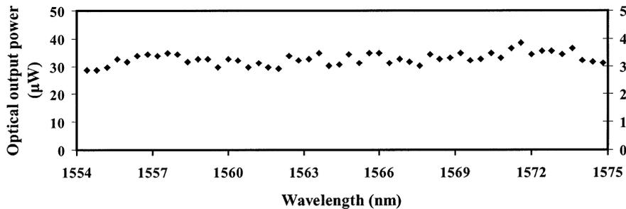
WJ2 Fig. 3. Power distribution in output wavelength channels.
