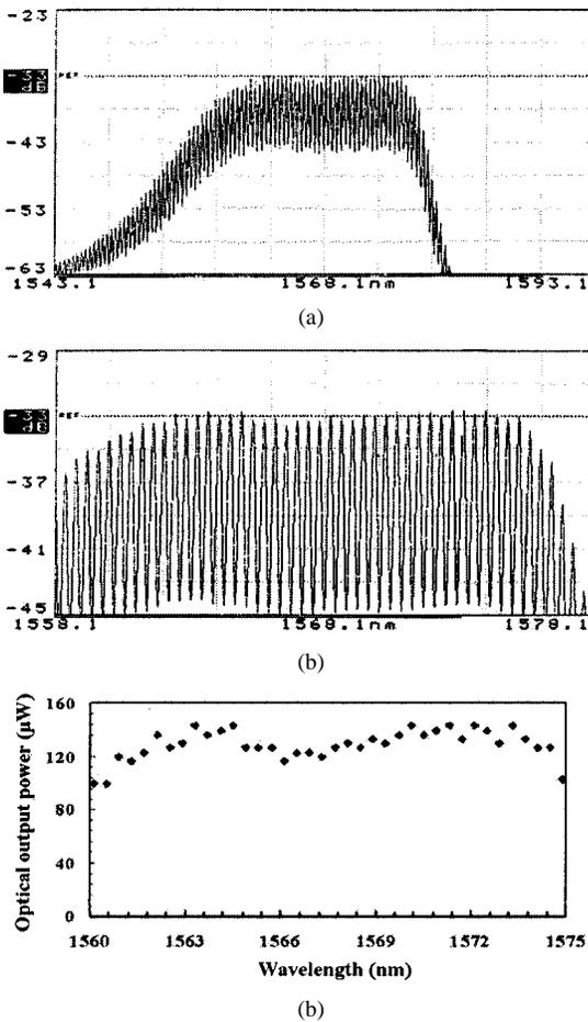
Fig. 2. Optical spectrum at (a) sweep width 5 nm/div (b) sweep width 2 nm/div, and (c) power distribution of output wavelengths.
