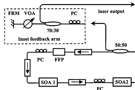
Fig. 1. Experimental setup and inset showing the feedback arm.
