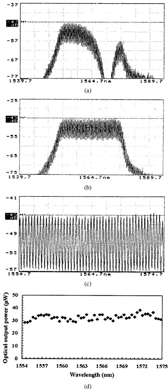
Fig. 3. Optical spectrum: (a) without and (b) with optical feedback (sweep width 5 nm/div). (c) With optical feedback (sweep width 2 nm/div). (d) Power distribution of output wavelengths with feedback.
