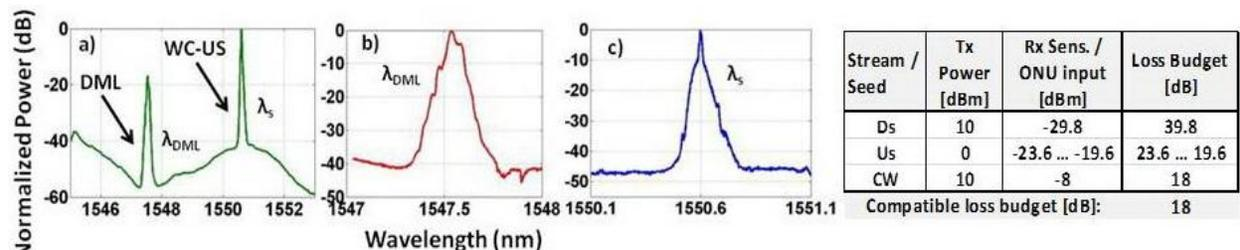
**Figure 4:** Spectra of a) AOWC output, b) upstream signal, and c) DML output. The table summarizes the compatible B2B loss budgets.
