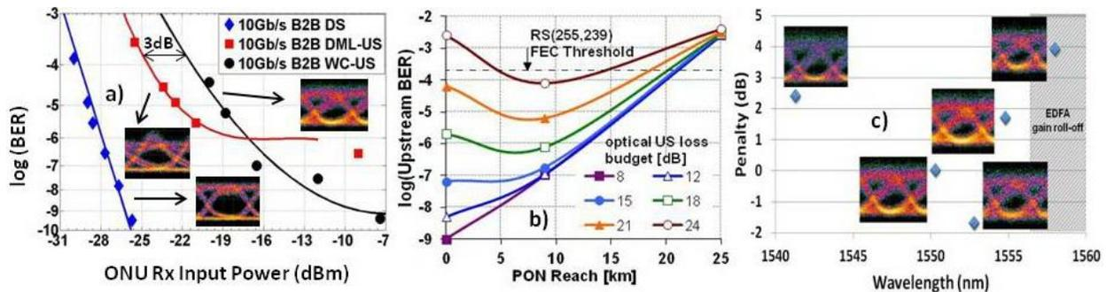
**Figure 3:** BER for a) B2B downstream and upstream with DML and DML+WC, b) compatible PON reach for the upstream after AOWC for various loss budgets, and c) colorless operation of the AOWC showing the penalty with respect to 1550.3 nm.
