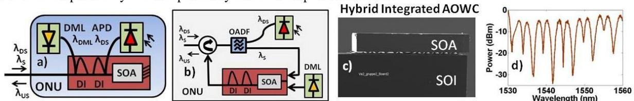
**Figure 1:** a) proposed ONU scheme, b) proof-of-principle ONU, c) SEM image of fabricated AOWC, d) spectral DI response for ASE seed
