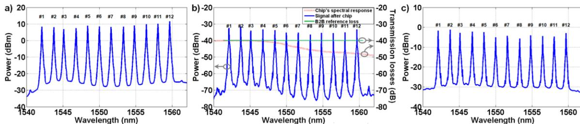
Fig. 2. Spectra of the 12x40 Gb/s WDM signal a) at chip’s input, b) at chip’s output, in comparison with chip’s spectral response and B2B flat losses, c) after post-chip amplification
