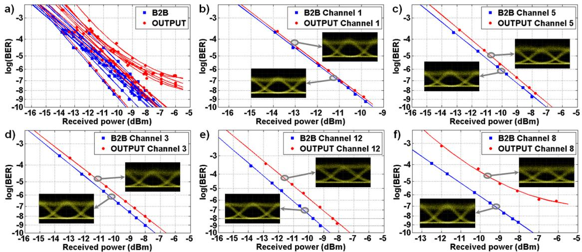
Fig. 3. BER curves for a) all 40 Gb/s B2B and transmitted channels, b) ch. #1, c) ch. #5, d) ch. #3, e) ch. #12, f) ch. #8
