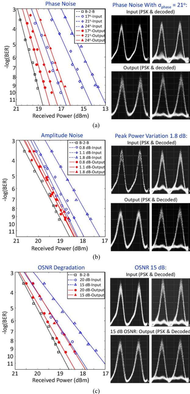
Fig. 5. Experimental results for input signals with (a) phase-, (b) amplitude-, and (c) ASE noise. The left panel summarizes the BER measurements for various  $\sigma_{\text{phase}}$ , peak power variation, and OSNR values at the input, respectively. The right panel depicts eye-diagrams of the PSK and the decoded signals at the input and output of the regenerator in selected cases.
