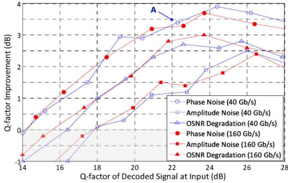
Fig. 2.  $Q$ -factor improvement of the decoded signals after the regenerator for different types of signal degradation at 40 and 160 Gb/s.
