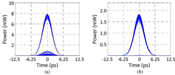
Fig. 3. Eye-diagrams of the 40-Gb/s decoded signal at the (a) input, and (b) output of the regenerator. The eye-diagrams correspond to point A in Fig. 2.
