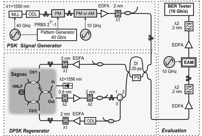
Fig. 4. Experimental setup at 40 Gb/s.
