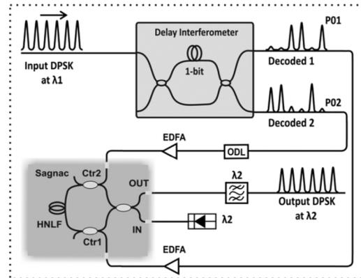
Fig. 1. Operating principle of the fiber-based DPSK regenerator and wavelength converter.
