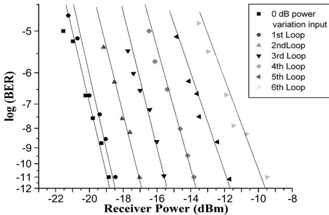
Fig. 3. BER measurements after each loop transit.
