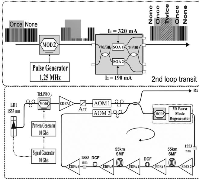
Fig. 1. (a) Graphic representation of the circulating signal for the second loop transit. (b) Loop experimental setup.
