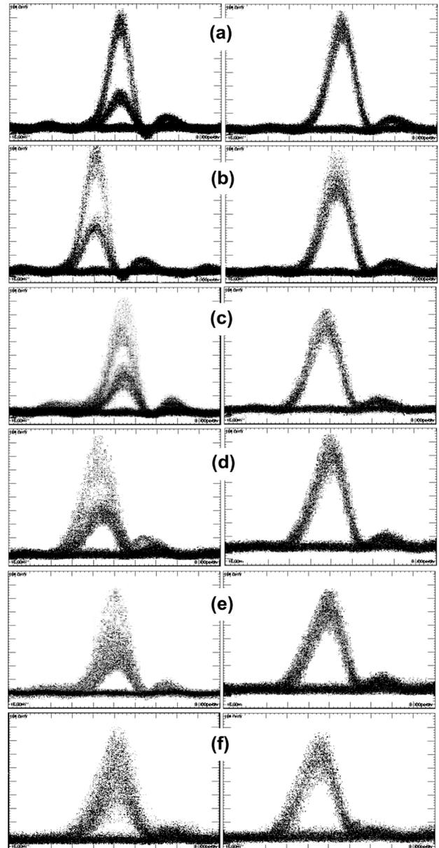
Fig. 2. Input and output signal eye diagrams for (a) first, (b) second, (c) third, (d) fourth, (e) fifth, and (f) sixth loop transit. The time scale is 8 ps/div.
