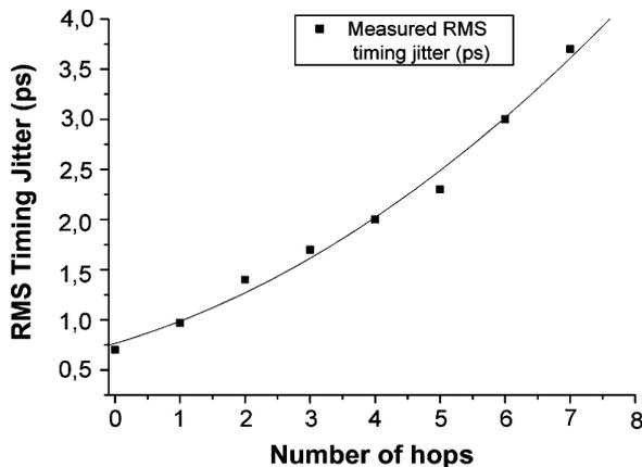
Fig. 4. Measured rms timing jitter for seven consecutive loops.
