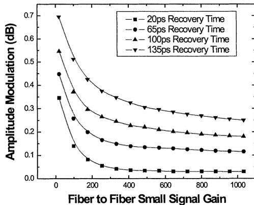
Fig. 4. Amplitude modulation versus SOA small-signal gain for various recovery times.
