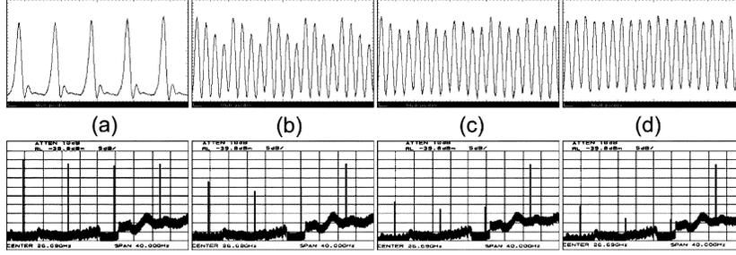
Fig. 2. Oscilloscope traces and corresponding RF spectra at the (a) compressor output, (b) Fabry–Perot filter output, (c) output after first SOA pass, and (d) output after second SOA pass. Oscilloscope trace time base is 50 ps/div. Microwave spectra amplitude scale is 5 dB/div and frequency scale is 4 GHz/div.
