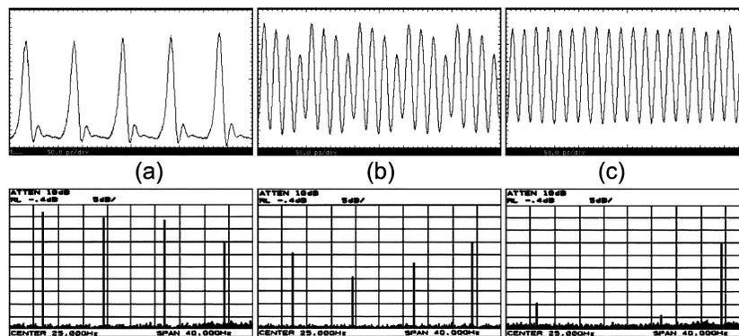
Fig. 7. Oscilloscope traces and corresponding microwave spectra (a) at the compressor output, (b) after the first pass through the FP filter, and (c) after the second pass through the FP filter. The oscilloscope trace time base is 50 ps/div. The microwave spectra amplitude scale is 5 dB/div and the frequency scale is 4 GHz/div.
