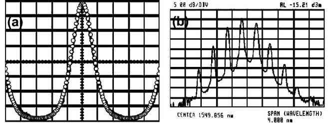
Fig. 3. (a) Second-harmonic autocorrelation trace. The white dots indicate the fitted hyperbolic squared-secant periodic autocorrelation profile. The time base is 2.74 ps/div. (b) Optical spectrum trace. The amplitude scale is 5 dB/div and the frequency scale is 0.4 nm/div. The resolution 0.08 nm.
