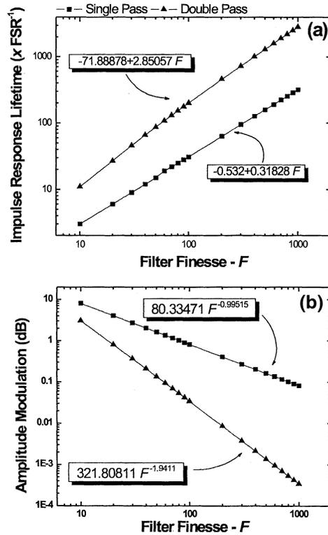
Fig. 10. (a) Calculated impulse response  $1/e$  lifetime versus FP filter finesse. (b) Calculated amplitude modulation versus FP filter finesse, in the single and double pass cases.
