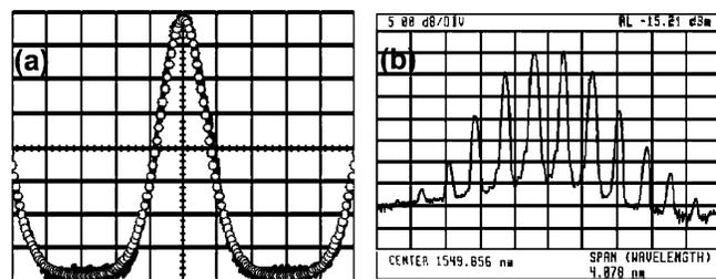
Fig. 8. (a) Second-harmonic autocorrelation trace. The white dots indicate the fitted hyperbolic secant periodic autocorrelation profile. Time base is 2.74 ps/div. (b) Optical spectrum trace. The amplitude scale is 5 dB/div and the frequency scale is 0.4 nm/div. Resolution 0.08 nm.
