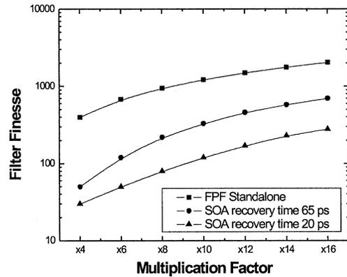
Fig. 5. Calculated filter finesse versus desirable pulse repetition frequency under the constraint that amplitude modulation remains close to 0.2 dB, for SOAs with recovery time equal to 20 ps, 65 ps, or no SOA.
