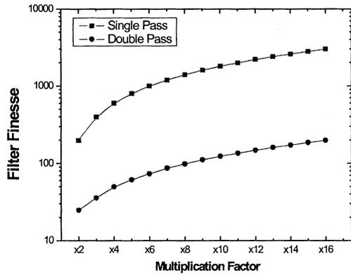
Fig. 11. Required filter finesse versus desirable pulse repetition frequency for the single- and double-pass cases under the constraint that amplitude modulation remains under 0.14 dB.
