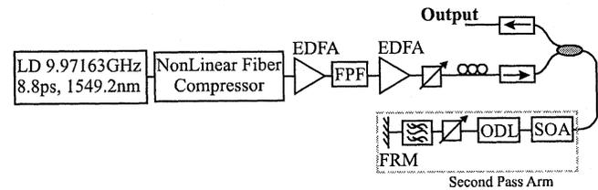
Fig. 1. Experimental setup. ODL: optical delay line; FRM: Faraday rotator mirror.
