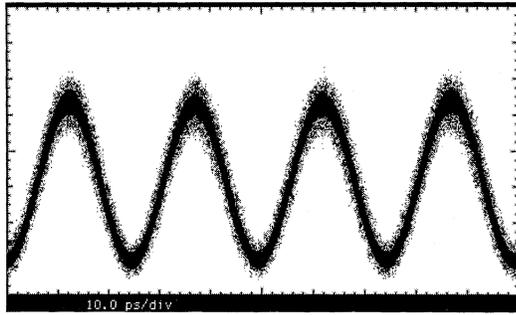
Fig. 9. Waveform of the output 40-GHz pulse train. The time base is 10 ps/div.
