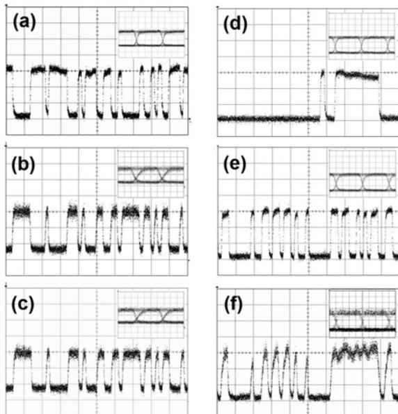
Figure 2: (a), (b), (c) Read mode operation: (a) inverted Access bit, (b) Read output at  $\lambda_0$ , (c) Read output at  $\lambda_1$ . (d), (e), (f) Write mode operation: (d) inverted Access bit, (e) incoming *Bit*, (f) RAM cell memory content recorded at S/P1 ( $\lambda_1$ ). Time scale: 1ns/div for traces, 50ps/div for the eye diagrams shown in the insets.
