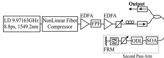
Fig. 1. Experimental Setup.
