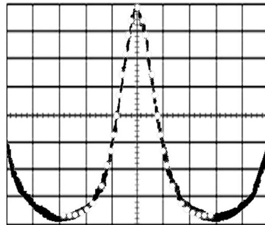
Fig. 3. Second-harmonic autocorrelation trace. The white dots indicate the fitted hyperbolic secant autocorrelation profile. Time base is 3.66 ps/div.
