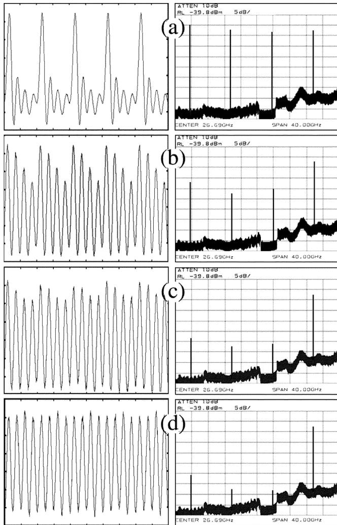
Fig. 2. Oscilloscope traces and corresponding radio-frequency (RF) spectra at the (a) compressor output, (b) FPF output, (c) output after first SOA pass, and (d) output after second SOA pass. Oscilloscope trace time base is 50 ps/div. RF spectra amplitude scale is 5 dB/div and frequency scale is 4 GHz/div.
