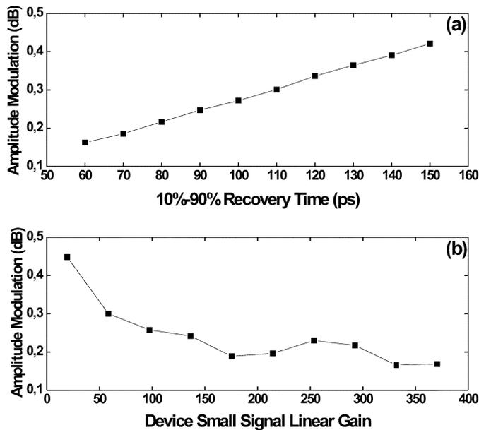
Fig. 4. (a) Amplitude modulation versus SOA recovery time and (b) amplitude modulation versus device small-signal gain.
