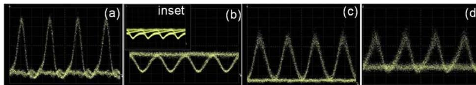
Figure 2 : Experimental results: a) input signal, b) inverted WC, inset inverted signal at the output of the SOA c) WC signal after DI and d) non-inverted WC. Time scale is 10 ps/div.
