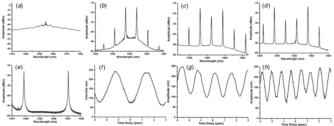
**Figure 3.** Experimental results. (a) Supercontinuum spectrum at the output of the HNLF (span: 50 nm), (b)–(e) generated optical spectra, spaced at (b) 396 GHz (span: 20 nm), (c) 792 GHz (span: 20 nm), (d) 1.188 THz (span: 20 nm) and (e) 2 THz (span: 25 nm). (f)–(h) optical autocorrelation traces of the DFG source at (f) 396 GHz, (g) 792 GHz and (h) 1.188 THz.
