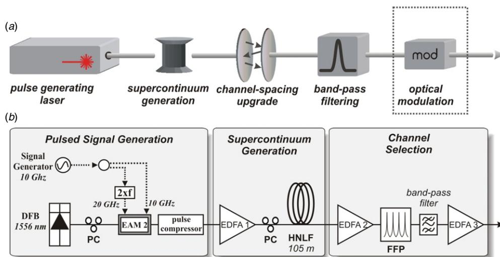
Figure 2. (a) Block diagram and (b) experimental setup for the tunable-DFG source. PC: polarization controller, 2xf: electronic frequency doubler.
