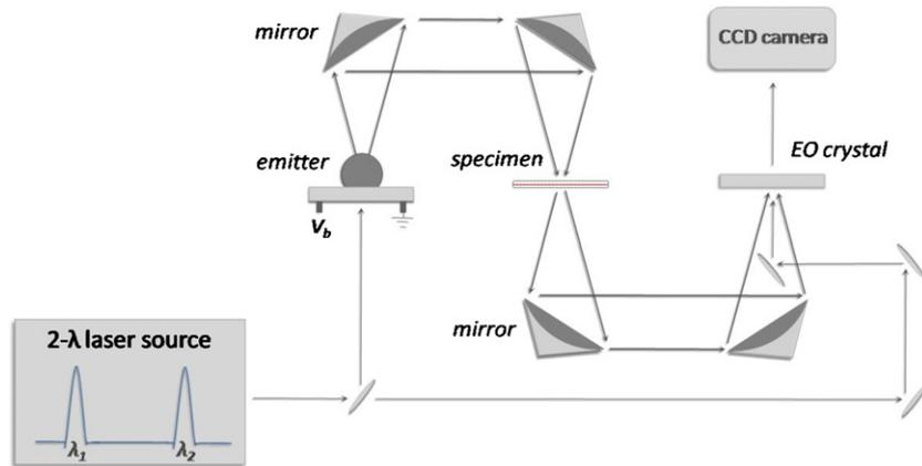
Figure 1. Block diagram of the 2D THz imaging system.
