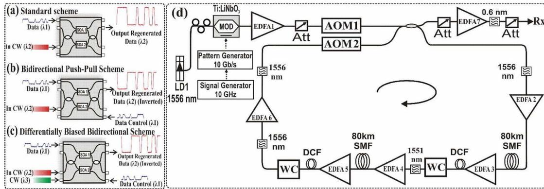
Fig. 1. Principle of operation of (a) standard WC scheme with one control signal, (b) bidirectional push-pull WC scheme, and (c) differentially biased bidirectional push-pull scheme with additional CW signal. (d) Experimental loop setup.
