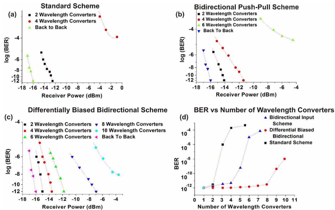
Fig. 3. BER measurements.
