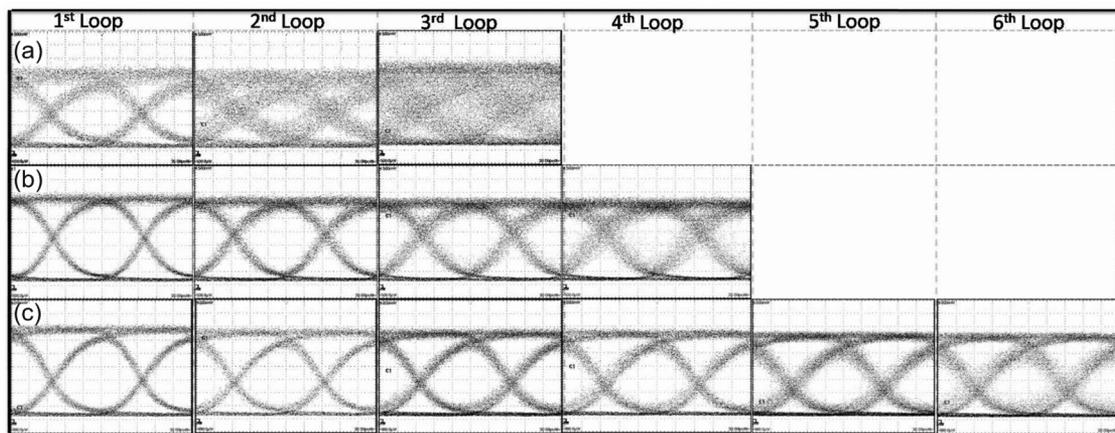
Fig. 2. Eye diagrams at the loop output for (a) standard WC scheme with one control signal, (b) bidirectional push-pull scheme, (c) differentially biased bidirectional push-pull scheme. Each loop employs two cascaded wavelength converters in sequence. Eye-diagram time scales are 20 ps/div.
