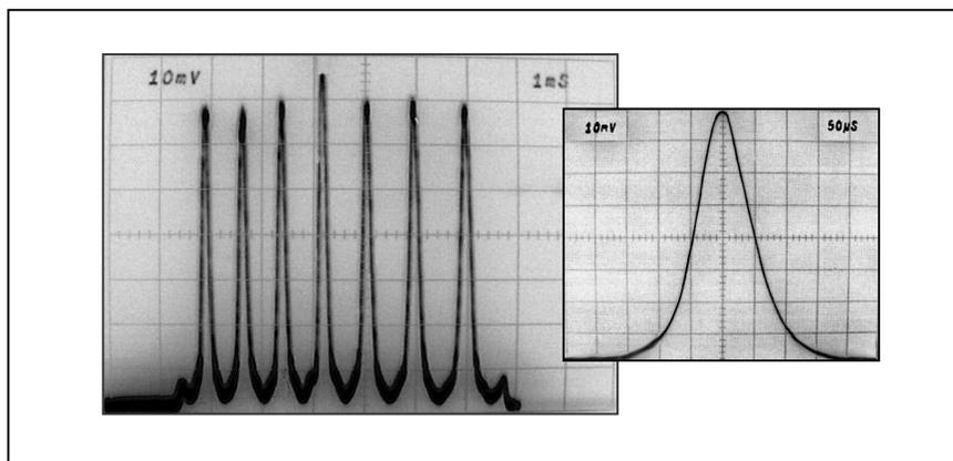
Figure 2: Autocorrelation of the 2.2 ps, 40 GHz pulse train after the fiber compressor.
