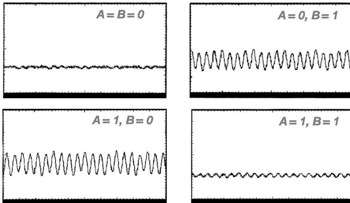
Figure3: Switched port outputs for the four logical combinations of clock A and B. The time-base is 50 ps.
