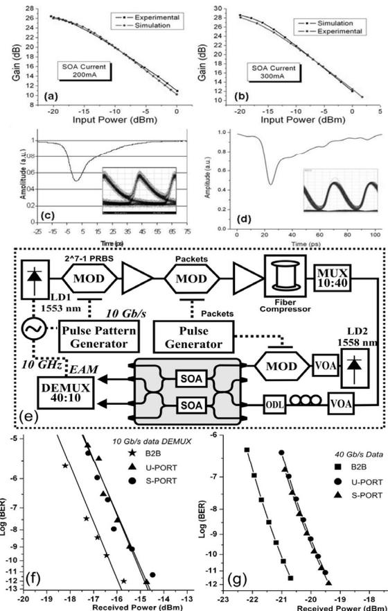
Figure 2 : Comparison between simulation and experimental results. SOA gain response when operated at (a) 200 mA and (b) 300 mA. Recovery time measurements (c) provided by supplier and (d) using the simulation model. Insets show corresponding 10 Gb/s wavelength conversion. Experimental setup (e) and experimental (f) versus simulation (g) BER curves (g) for 40 Gb/s packet switching.
