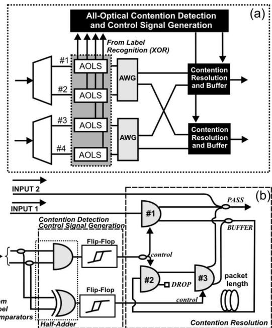
Figure 1 : (a) AOLS node architecture based on optical label processing and internal non-blocking wavelength routing and (b) logical design diagram of all-optical contention detection and resolution.
