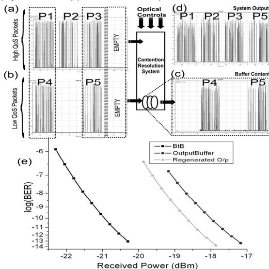
**Figure 3 : (a-d) Time-domain traces for the simulated scenario: a) high priority incoming packets, b) low priority incoming packets, c) buffer content and d) output of the system. e) Simulation BER results for back-to-back and output of the system before and after 2R regeneration.**
