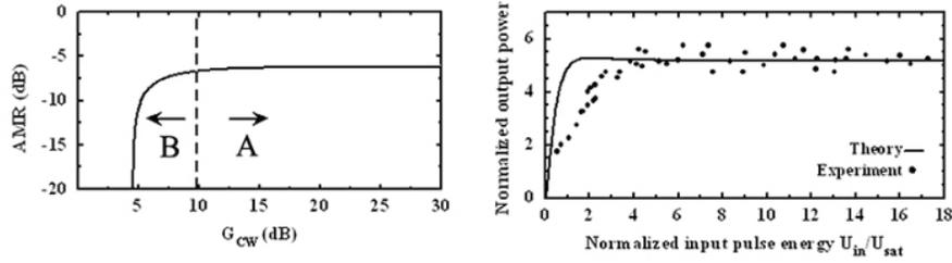
Fig. 3. (a): Amplitude modulation reduction (AMR) vs the steady-state gain value  $G_{CW}$  of the SOA that describes its saturation level (b): experimental and theoretical power transfer function.
