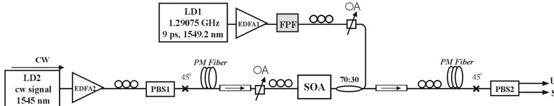
Fig. 1. Experimental setup. FPF: Fabry-Perot filter, OA: optical attenuator, PC: Polarization Controller, PBS: Polarization Beam Splitter, PM Fiber: Polarization Maintaining Fiber
