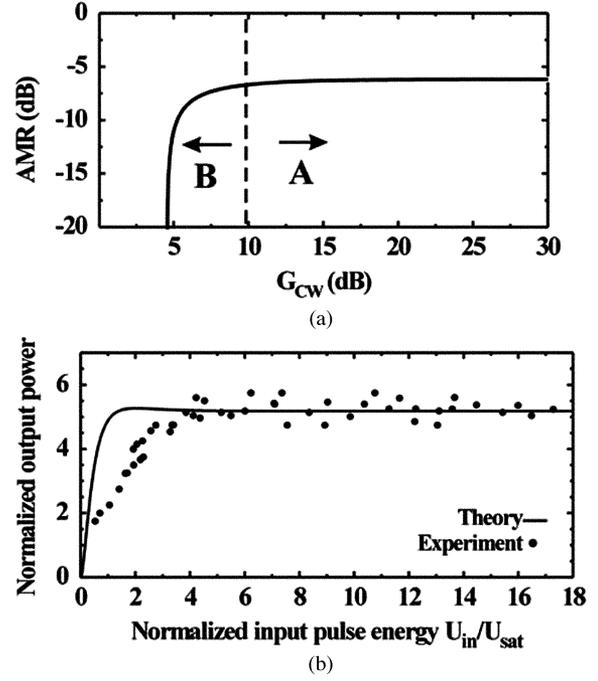
Fig. 2. (a) Theoretically calculated AMR at the output of the MZI gate for various  $G_{CW}$  values. (b) Theoretical (solid line, for  $G_{CW} = 2.85$ ) and experimental (black circles) power-limiting output power versus input pulse energy transfer function.
