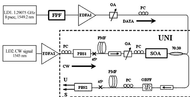
Fig. 3. Experimental setup. OA: optical attenuator. PC: polarization controller. PBS: polarization beam splitter. OBPF: optical bandpass filter. PMF: polarization-maintaining fiber.
