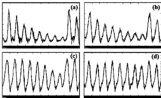
Fig. 4. (a) Control pulse sequence at the FPF output, (b), (c), (d) corresponding switched pulse trains at the output of the gate for a control power of (b) 200, (c) 600, and (d) 800  $\mu$ W. Time base: 100 ps/div.
