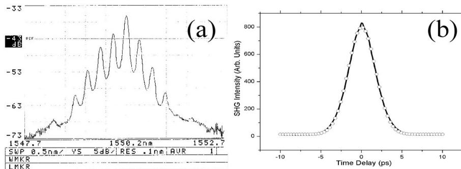
Fig. 4. Recovered clock (a) optical spectrum and (b) autocorrelation trace with sech fitting.
