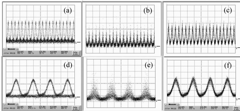
Fig. 3. Eye diagrams of (a) incoming data, (b) FPF output and (c) extracted clock at 50 ps/div and (d) incoming data, (e) FPF output and (f) recovered clock at 10 ps/div. The vertical scale of upper row is  $390\mu\text{W}/\text{div}$  and the lower row vertical scale is  $500\mu\text{W}/\text{div}$ .
