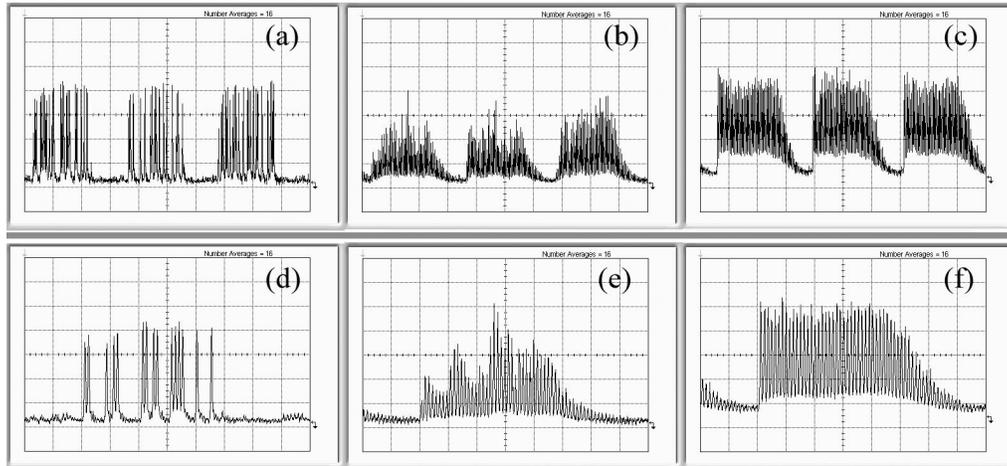
Fig. 2. Pulse traces of (a) three input data packets, (b) corresponding FPF output, (c) recovered clock packets at time base 500 ps/div and (d) single packet, (e) FPF output and (f) single recovered clock packet at time base 200 ps/div. The vertical scale is 335 μW/div.
